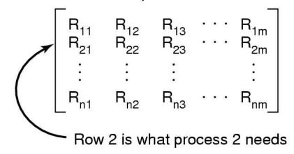
Data structures needed by deadlock detection algorithm
