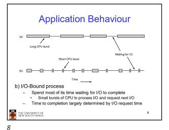
Observation Long CPU burst Waiting for I/O We need a mix of CPU-bound and I/O-bound processes to keep both CPU and I/O systems busy Process can go from CPU- to I/O-bound (or vice versa) in different phases of execution THE UNIVERSITY OF NEW SOUTH WALES
