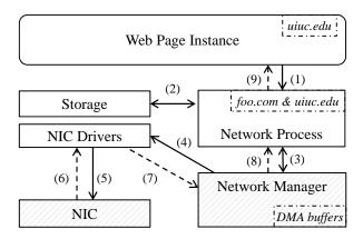
Figure 2: This figure enlarges the right half of Figure 1 and shows how our IBOS subsystems interact when a web page instance from uiuc.edu issues a network request to foo.com. Subsystems are shown in boxes and solid and dotted arrows represent IBOS messages for outgoing and incoming data respectively. The reference monitor (which is not shown here) checks all these messages to enforce security properties.
