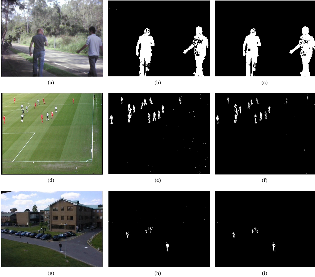
Figure 5. Sample background subtraction outputs for MoG (middle column) and CS-MoG-Balanced (rightmost column). The i -th ( i = 1, 2, 3 ) row contains the results from the i -th dataset. The original frames are in the leftmost column.
