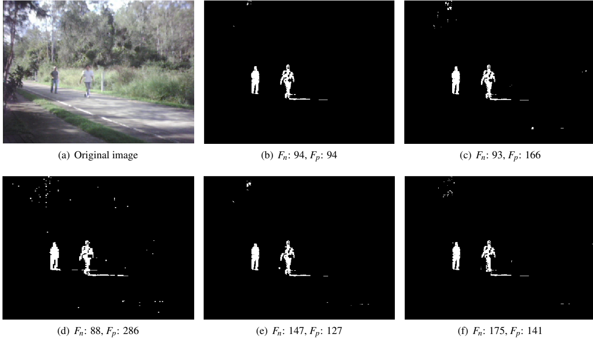
Figure 6. Sample background subtraction output for various MoG based methods. (a) Original frame, (b) CS-MoG-Balance, (c) CS-MoG-Unbalance, (d) Original MoG, (e) Mean-MoG, (f) RS-MoG.
