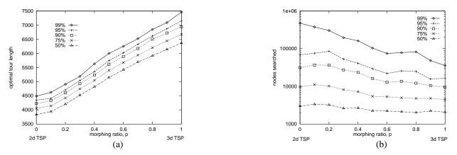
**Figure 5.** Percentiles in (a) optimal tour length and (b) cost to find optimal tour for 20 city TSP problems constructed by morphing between two and three dimensions. In the 3-d case, cities are distributed uniformly and at random within a cube of side 1000. In the 2-d case, we project the 3-d problems down onto the x-y plane. Each data point is the average of 1000 problems.
