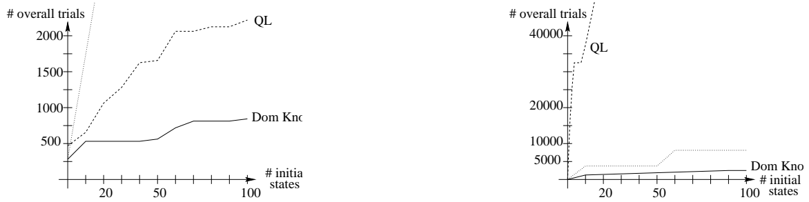
Figure 2: The charts show the overall number of trials before the n^{\text{th}} initial system state was managed to be balanced. The left chart shows the results for the state space based on 10 intervals per variable, i.e. 10 000 states. The right chart shows the results for the state space based on 25 intervals per variable respectively, i.e. 390 625 states. The solid lines show the results with the use of domain knowledge. The dashed lines show the Q-Learning results. The dotted lines give the results for Q-learning with the small state space of 162 states for comparison.
