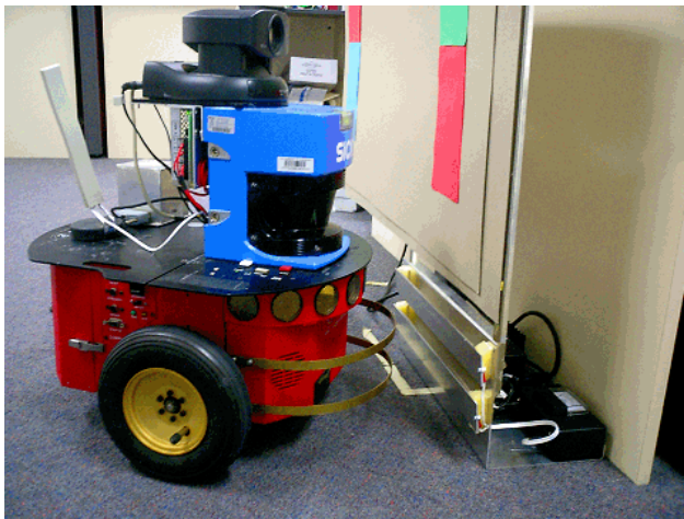
Figure 10: Photo of the rails mounted on the robot, entering the docking station.
