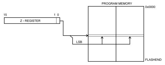
Constant byte address is specified by the Z-register contents. The 15 MSBs select word address. For LPM, the LSB selects low byte if cleared (LSB = 0) or high byte if set (LSB = 1). For SPM, the LSB should be cleared. If ELPM is used, the RAMPZ Register is used to extend the Z-register.
