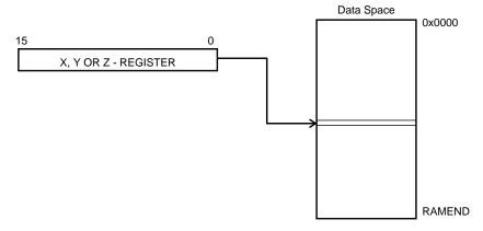
Operand address is the contents of the X-, Y-, or the Z-register. In AVR devices without SRAM, Data Indirect Addressing is called Register Indirect Addressing. Register Indirect Addressing is a subset of Data Indirect Addressing since the data space form 0 to 31 is the Register File.
