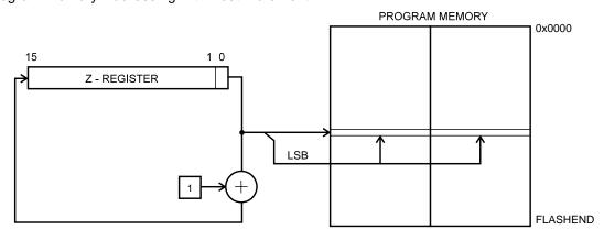
Constant byte address is specified by the Z-register contents. The 15 MSBs select word address. The LSB selects low byte if cleared (LSB = 0) or high byte if set (LSB = 1). If ELPM Z+ is used, the RAMPZ Register is used to extend the Z-register.
