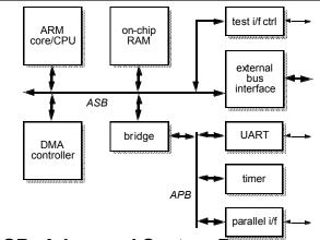
° ASB: Advanced System Bus: To connect High Performance modules
