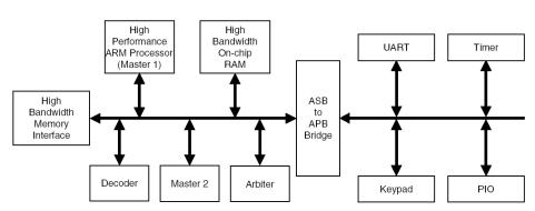
Need a Mechanism to allow various Processing units to access the Memory Bus without causing conflict
