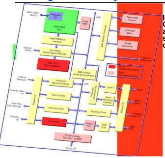
Integration of Core Processor and many subsystem microcells
