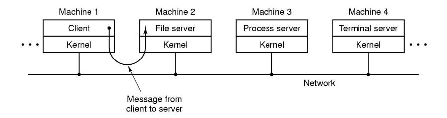
The client-server model of microkernel make it easier to extend to a distributed system
