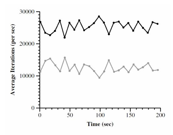
Figure 5: **Fairness Over Time.** Two tasks executing the Dhrystone benchmark with a 2:1 ticket allocation. Averaged over the entire run, the two tasks executed 25378 and 12619 iterations/sec., for an actual ratio of 2.01:1.
