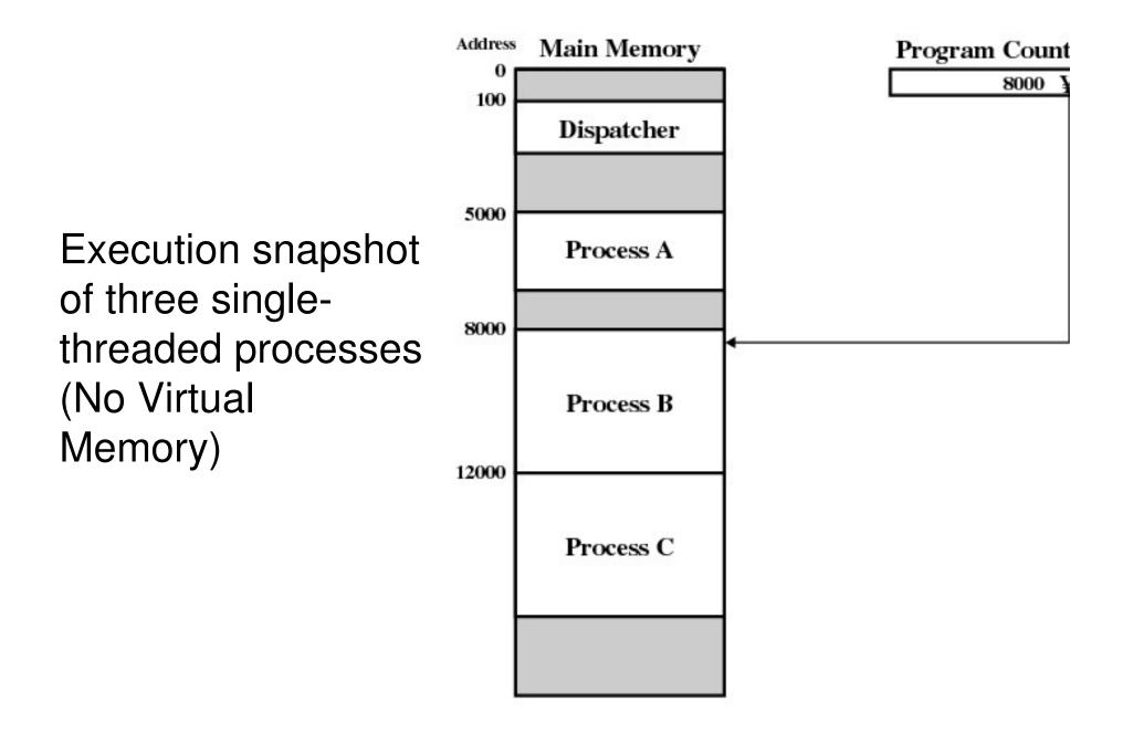
Figure 3.1 Snapshot of Example Execution (Figure 3 at Instruction Cycle 13
