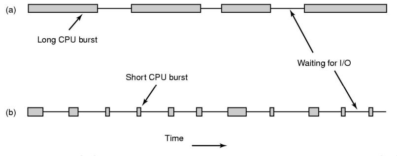
Bursts of CPU usage alternate with periods of I/O wait
