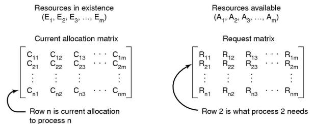
Data structures needed by deadlock detection algorithm
