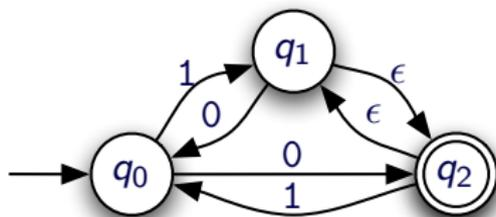
The input "001" is accepted. A possible run is  $q_0 q_2 q_1 q_0 q_1 q_2$ .
