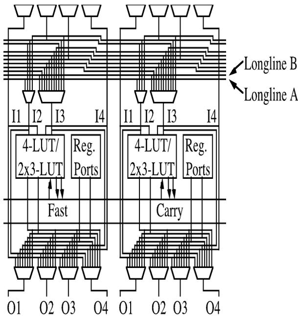
Fig. 2. Chimaera reconfigurable array routing structure (two cells within a row of the array).
