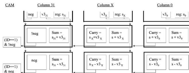
Fig. 7. RFU contents of the MPEG2 encoder example. The RFUOP selects from either the fourth or fifth row, depending on the value of the negative flag. This method saves an extra row, which otherwise would need to select from either the fifth or sixth row.
