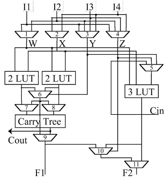
Fig. 3. Chimaera reconfigurable array logic block (the 4-LUT/2x3-LUT structure within Fig. 2).
