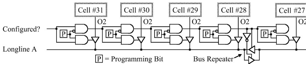
Fig. 4. Control logic for the longlines, including logic to avoid multiple writer conflicts and a repeater.
