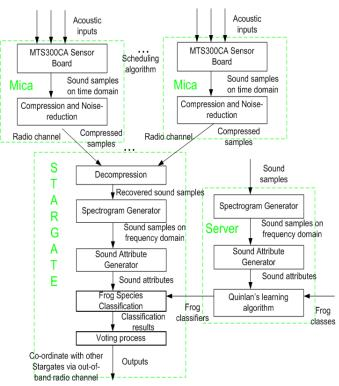
Fig. 6. The architecture of *Hybrid (Stargates and Mica2s)* system. In this system, instead of sampling acoustic data using desktop microphone, we use MICA2s to sample acoustic data, and compress it before sending to the Stargate via radio channel. Upon receiving data from the satellite motes, the Stargate will decompress received data before processing it.
