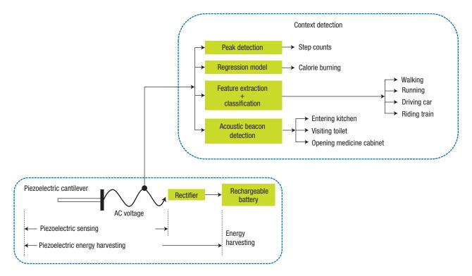
FIGURE 2. Converting energy to context in a piezoelectric energy harvester (PEH). The PEH uses kinetic energy harvesting to extract a range of health and lifestyle data without specialized motion sensors.
