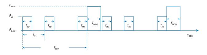
**FIGURE 4.** Power-consumption parameters of a duty-cycled system.  $T_{SI}$ : sampling interval;  $T_{MD}$ : time to read a sample;  $P_{MD}$ : average system power consumed during a sample reading from the sensor;  $T_{CDW}$ : length of one cycle of data collection;  $T_{RADIO}$ : time to transmit all data from one cycle;  $P_{RADIO}$ : radio power consumption;  $P_{SLEEP}$ : system power consumption during sleep.
