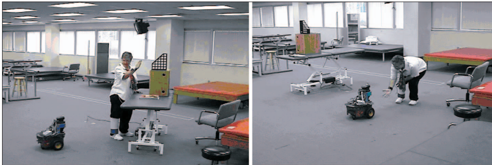
Figure 5. A stroke patient interacting with a socially assistive robot from Maja Matarić's lab that is monitoring, coaching, and motivating prescribed exercise therapy.
