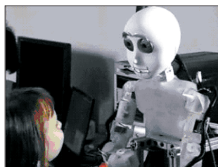
Figure 6. A child-sized humanoid robot, which Maja J. Matarić and her colleagues developed, interacts with a child. The robot works from a desktop or on a mobile platform and is an example of the research toward robots that can help in the education and socialization of children with special needs.
