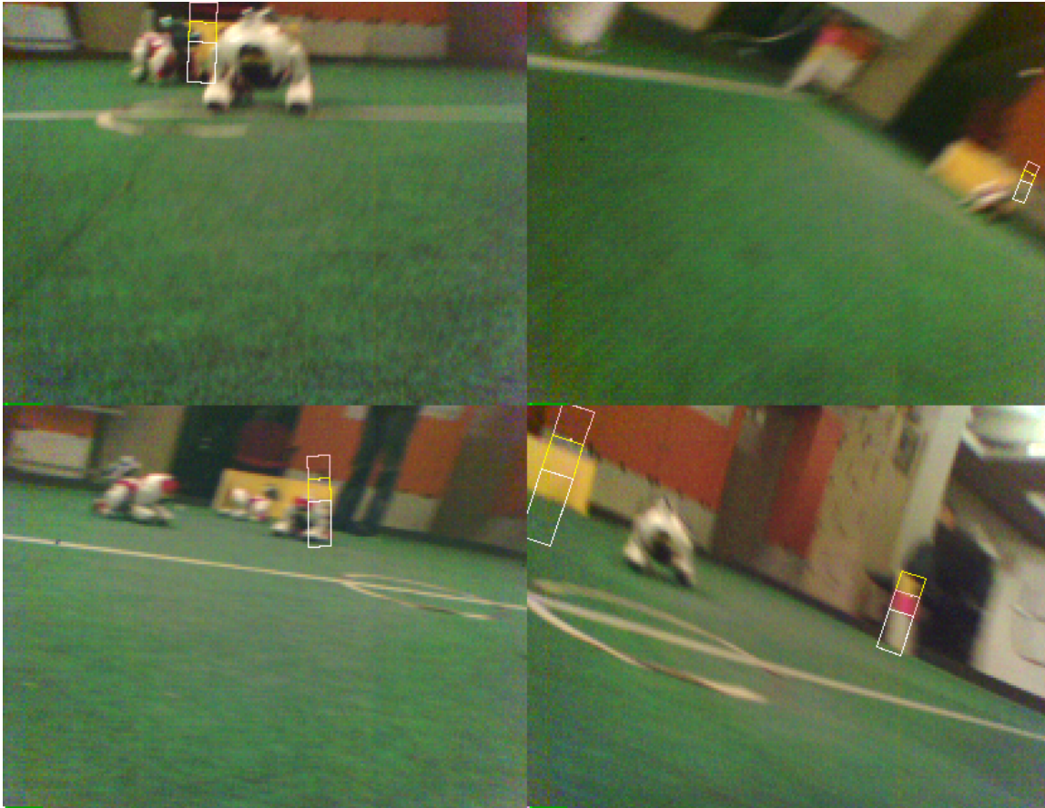
Figure 2.18: Some examples of false beacons being seen in the rUNSWift lab when pink and red are merged into one colour.
