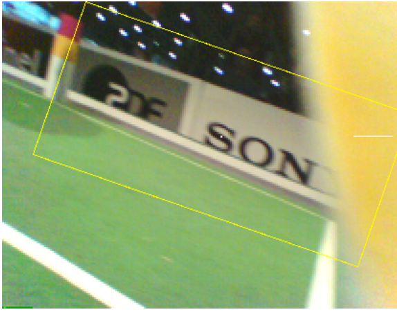
Figure 2.13: The misfit goal from the testing data in frame 71497. All three systems being tested misfit the goal in this way, however here the beacon is rejected due to the extra check added for the Merged system (in the other vision systems, this beacon was recognised).
