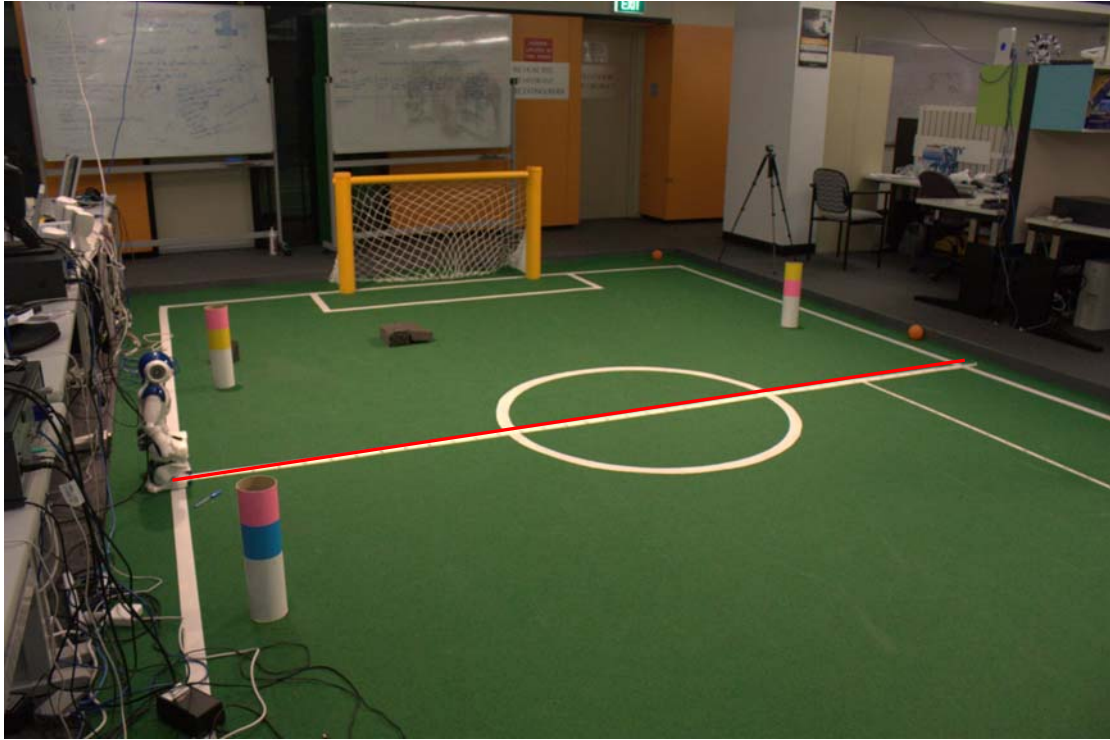
Figure 4.2: Field with Nao. The Nao was made to walk straight on the red line. The width of the field is 4.0m
