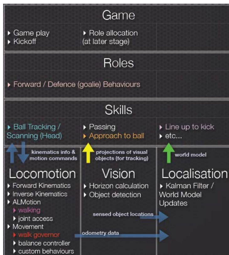
Figure 1.0: rUNSWift Architecture (Collien, D., Huynh, G.)
