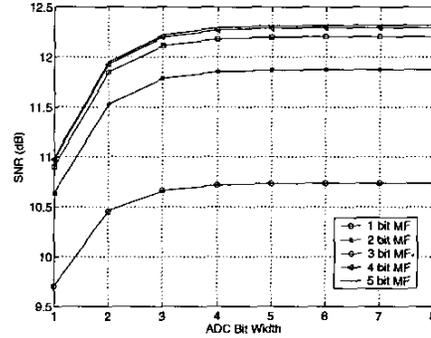
Figure 5: SNR vs ADC bit
