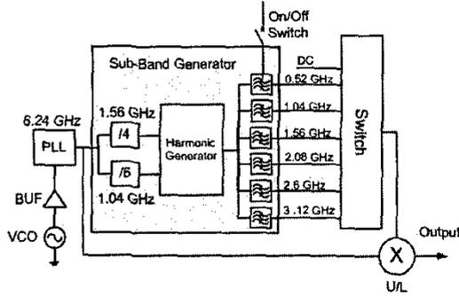
Figure 3: Multi-Frequency Generator
