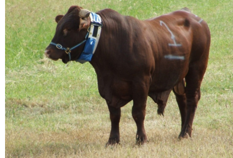
Figure 1: Photo taken during trial of bull wearing collar containing Fleck™ hardware, batteries and antennas. Note the number painted on side was to aid in visual identification of bulls during the trial.
