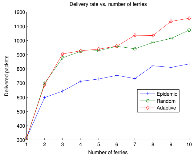
Figure 3. Performance of three different DTN protocols as number of ferries (animals) are varied.
