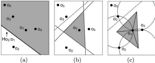
Figure 2: Computing Voronoi cell of  $o_1$
