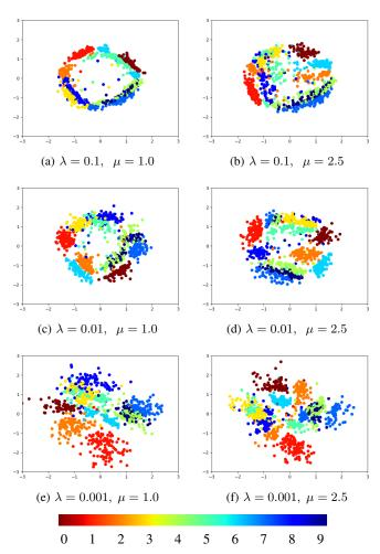
Fig. 3. Distribution in latent space of a random selection of test items, for Eccentric Autoencoder trained on the MNIST dataset using two latent dimensions, with  $\lambda=0.1,\,0.01$  or 0.001 and  $\mu=1.0$  or 2.5. The horizontal and vertical axes are the principal components corresponding to the larger and smaller eigenvalue of the covariance matrix.
