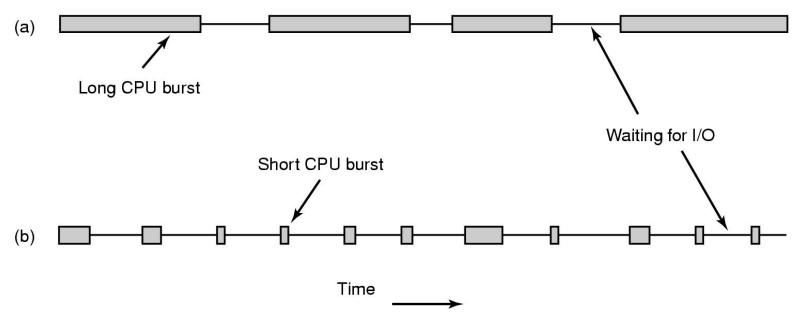
Bursts of CPU usage alternate with periods of I/O wait
