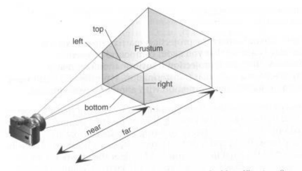
Figure 3-13 Perspective Viewing Volume Specified by glFrustum()
