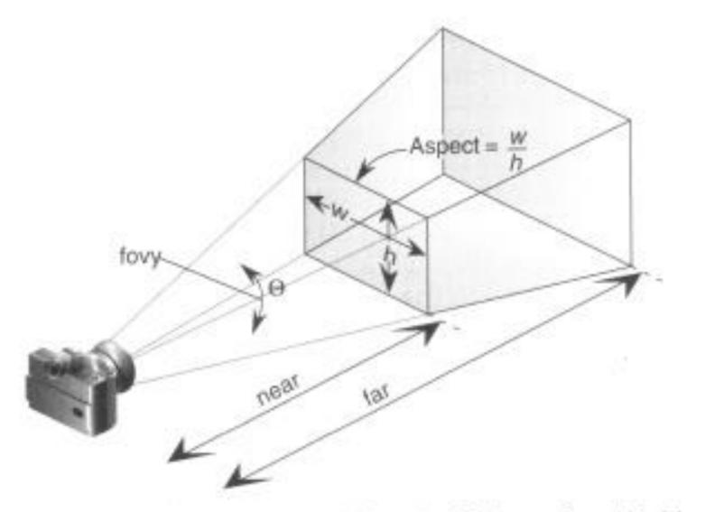
Figure 3-14 Perspective Viewing Volume Specified by gluPerspective()
