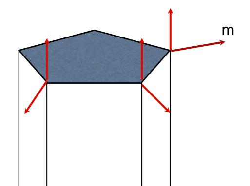
Illumination values are attached to each vertex and carried down the pipeline until we reach the fragment shading stage.
