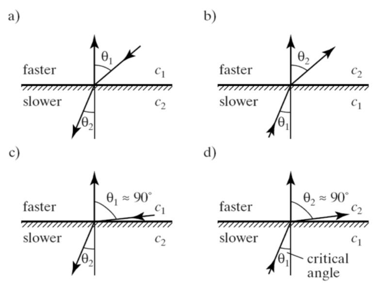
In (c) and (d), the larger angle has become nearly 90°. The smaller angle is near the critical angle: when the smaller angle (of the slower medium) gets large enough, it forces the larger angle to  $90^{\circ}$ . A larger value is impossible, so no light is transmitted into the second medium. This is called total internal reflection.
