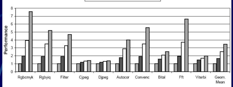
Figure 7. The performance of the VIRAM processor as a function of the number of vector lanes.
