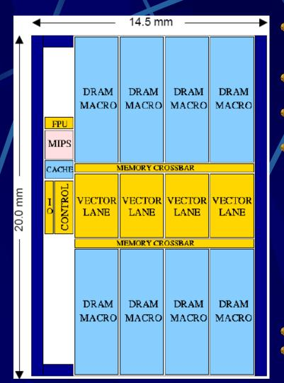
DRAM – Dynamic RAM – information must be periodically "refreshed" to mimic the behaviour of static storage On-chip DRAM connected to vector execution lanes via memory crossbars c.f. most SRAM cache-based machines – SRAM is more expensive, less dense In conventional architectures:
