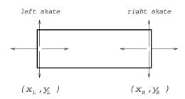
a skate at each end of the vehicle with which it can push on the rink in two independent directions
