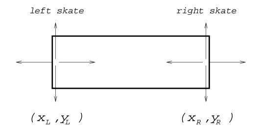
a skate at each end of the vehicle with which it can push on the rink in two independent directions
